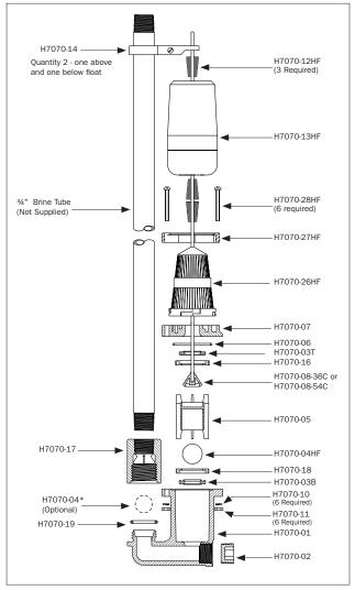
**NOTE:** The 454 %" High Flow Brine Valve is designed for salt brine only. It will also fit inside a brine well that is 5" or larger.
