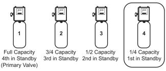
7. The primary tank regenerates. The next tank with the least remaining volume becomes the new primary tank. The tank with the next least volume remaining will be the first trip point programmed rate. Tanks continue operating in this order.
