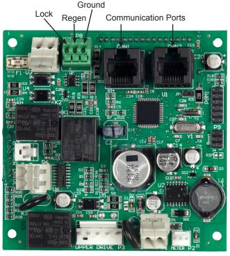
Figure 2 Current NXT Circuit Board
