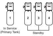
The total flow rate to the primary tank increased past the first trip point programmed rate. The flow stayed past the trip point delayed time. The next tank (least volume remaining) changes from Standby to In Service. This then splits the total flow between two meters.
