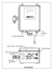
\*NOTE: Drill as required. These holes will only be drilled at factory if required.
