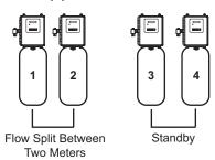
Tanks return to Standby due to decreased total flow rate and trip points programmed. The tank with the most remaining volume will be the first to go into Standby.
